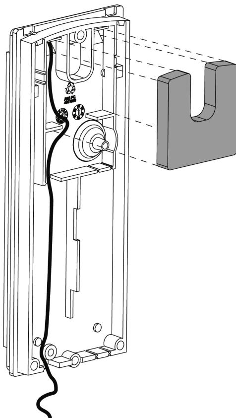
11. Place the detector on the mounting bracket from top side down and then lock the screw at the bottom.
