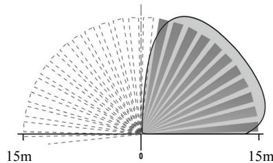
In order to change the detection beam direction rotate the internal detection element housing to the desired direction.
