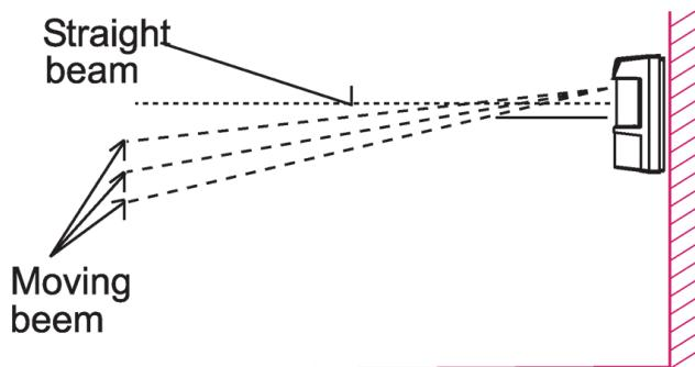
Changing the detection range is achieved by sliding the upper detection element up or down.
