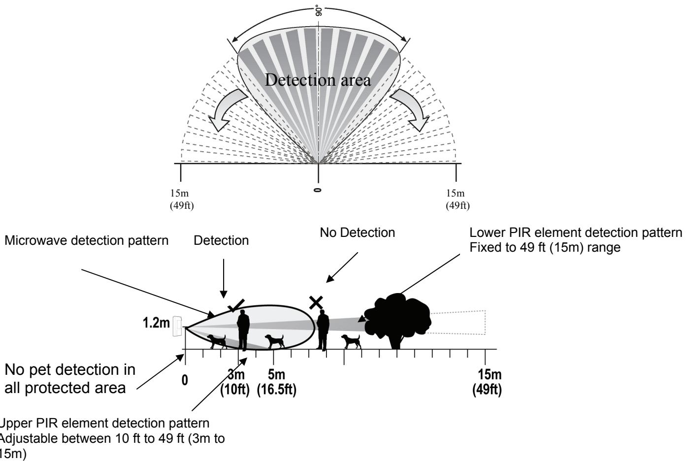
The EDS-3000 can differentiate between pets and human bodies and alert accordingly by having MW movement detection combined with two PIR detection beams:
