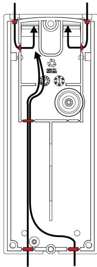
10. Attach the sealing "U" shaped Sponge Pad to the wire opening from the rear side after the wires connection and prior to final product affixing to the mounted bracket.
